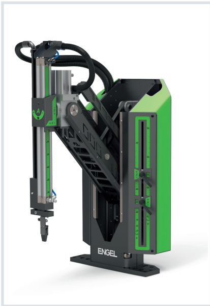
Fig. 1. The swivel arm replaces the fixed X-axis.
